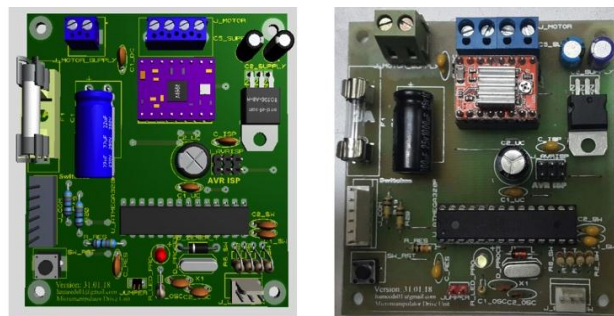
Fig. 4. Motor Drive Unit 3D animated view and fabricated board
